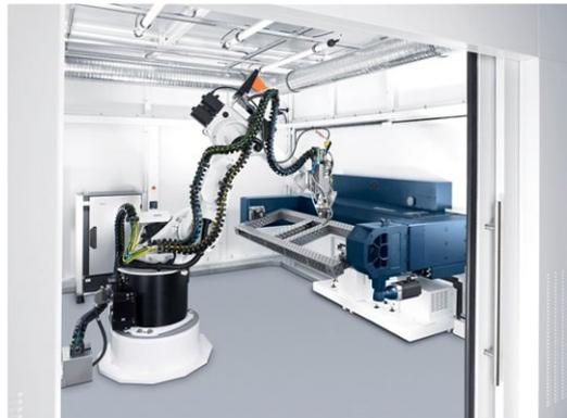
Parts with a weight of up to 750kg and a length of up to 2m can be easily positioned by means of the rotation changer.
